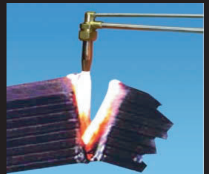
Cutting 8 layers steel sheet
